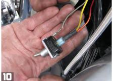
Plug the new connector onto the back of the switch. Make sure it's secure. Then reinstall the switch in the left triple tree cover.
