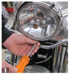
After putting a clean rag over your front fender, if you choose, remove the screw that holds the trim ring using a #2 Phillips screwdriver. Put the ring and screw aside for reinstallation later on.
