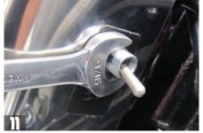
With the switch properly orientated in the cover, secure the switch using the stock nut and a 9/16" wrench. Then thread on the circular nut to lock it in place. Tighten it with the pliers.
