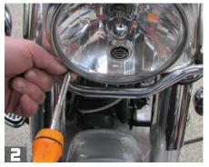
Then remove the three screws that hold the beauty ring to the headlight bucket using a #2 Phillips screwdriver. Set this ring and these screws aside for reinstallation later on.
