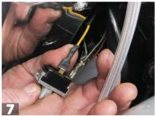
Pull the vellow wire (the one that's activated when this switch is turned on) from the back of the switch.
