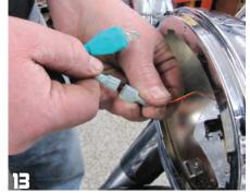
Join the two connectors you just installed. Some people like to then wrap some electric tape over the two connectors.
