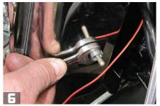
Use pliers to remove the circular nut and a 9/16" wrench to remove the hex nut that hold the stock spotlight switch to the triple tree cover. Then pull the switch (it's powered by the ignition switch) from behind the cover.
