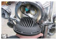
Align the three tabs on the back of the new Cyron headlight to the three notches in the stock headlight bucket.
